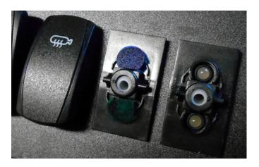
LEFT: Rocker switch cover shown installed and removed. Middle switch shows colored light filters installed. Right switch filters not installed, white LED lighting.
